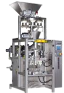
Vertical Bagger with Volumetric Cups Filler (For granulated Products)
