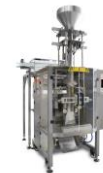
Vertical Bagger with Volumetric Cups Filler and inline labeler applicator (For granulated Products)
